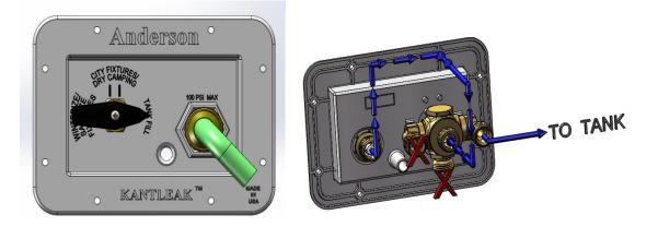
TO SANITIZE /WINTERIZE COLD FIXTURE (NOT TANK) FROM UNPRESSURIZED SOURCE (VIA RV PUMP)
