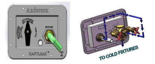
TO FILL STORAGE TANK FROM PRESSURIZED CITY WATER
